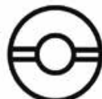
By-pass aperto Opened bypass
