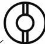
By-pass chiuso Closed bypass
