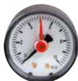
Manometro Ø 50 mm. Attacco 1/4" G posteriore o radiale. Pressure gauge 1/4", Ø mm 50, gas back or radial connection.
